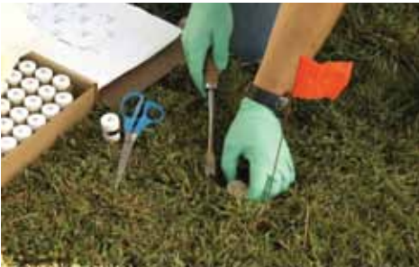
Remove cork by hand or with screwdriver.
