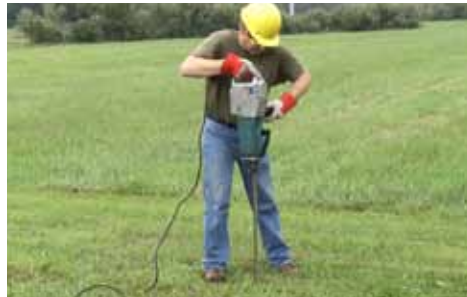
Rotary hammer drill and 36 in (1 m) long, 0.5 in (1 cm) diameter carbide-tipped bit
