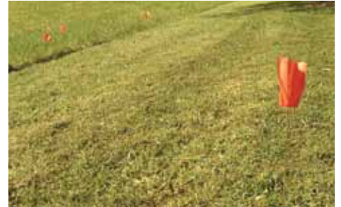
Lay out sampling grid prior to hole drilling.
