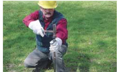
Hammer and 36 in (1 m) long, narrow diameter steel rod
