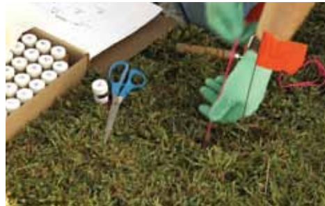
Pull string to remove sampler.
