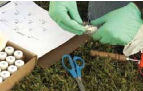
Return sampler to vial. Clean top of vial and threads, and secure cap.
