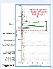
peaks in Figure 2 in the deltaic sandy shales of the Olmos Fm. Note the strong increase in the ratio between 2400 ft. and 3100 ft., once again implying seals at those two depths. The resistivity log also registered significant change between 2400 ft. - 3100 ft. This Sw proxy can be particularly helpful in fields, like the Woodford Shale, with high water saturation issues.
