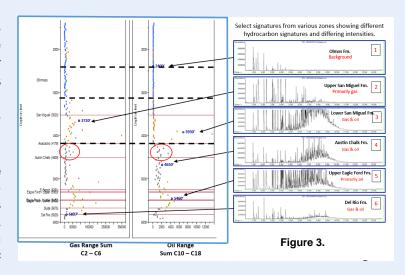
Miguel Fm. This implies a seal must be present between the two. The hydrocarbon profile showed hydrocarbons amassing at the seal at the top of the Anacacho Fm. (noted by the red circles). The hydrocarbon profile and the TIC also indicated a reduced hydrocarbon intensity or richness in the Austin Chalk and Anacacho Fms.
